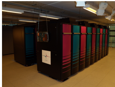
Figure: CSC (Center for Scientific Computing), Finland; Cray XT5/XT4 QC 2.3 GHz; Top500 Nov-2011 no. 202. Total cores: 10 864. Maximal performance R_{max} = 76,5 Tflop/s. Processors: Opteron Quad Core 4C 2.3 GHz. Processor technology: AMD x86_64.
