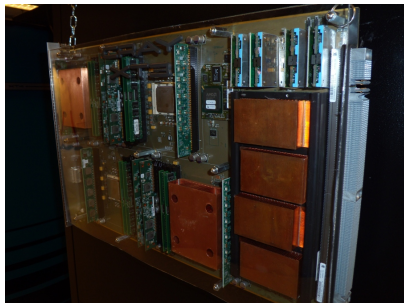
Figure: CSC (Center for Scientific Computing), Finland; Cray XT5/XT4 QC 2.3 GHz; Top500 Nov-2011 no. 202. Total cores: 10 864. Maximal performance R_{max} = 76,5 Tflop/s. Processors: Opteron Quad Core 4C 2.3 GHz. Processor technology: AMD x86_64.
