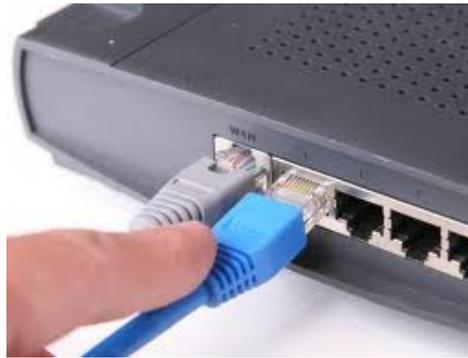
Figure 20. Connecting UTP cable to router
