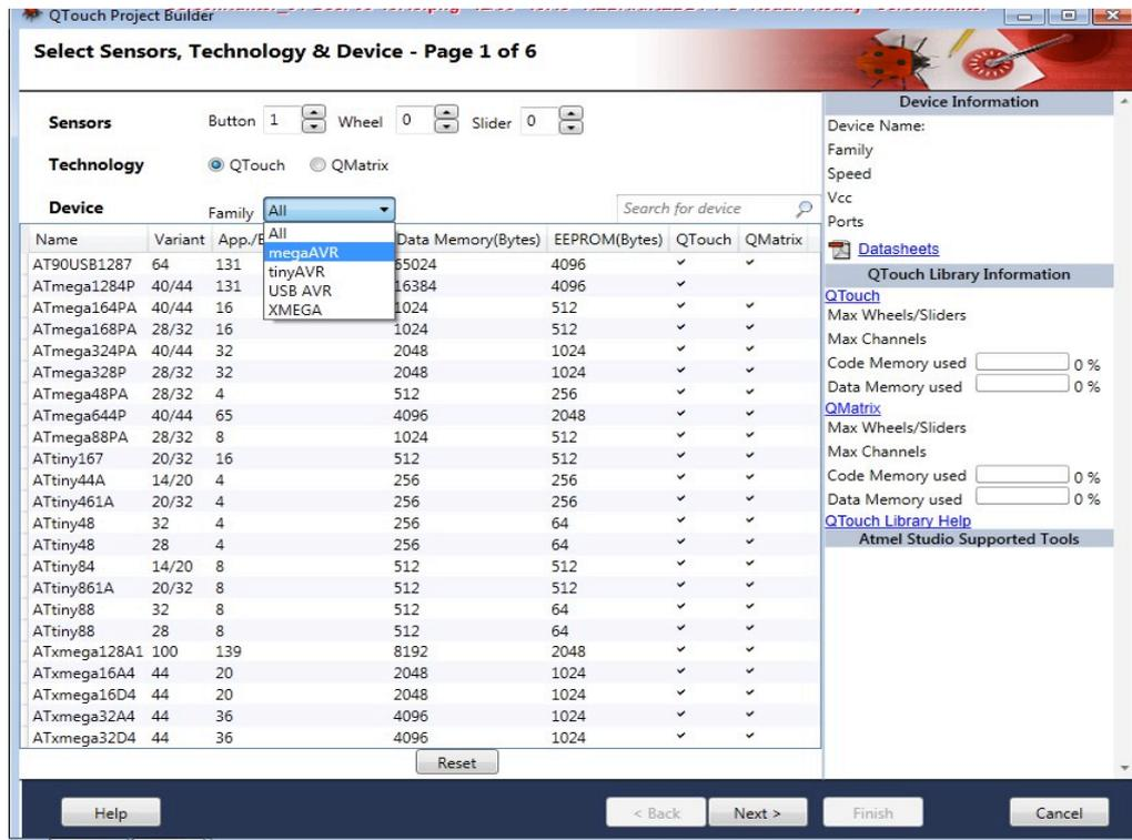
**Step 3 :** Select each sensor from the dropdown and assign a Sensor ID and define the size of each. The sensor ID assigned here will be used throughout to refer to the particular sensor.
