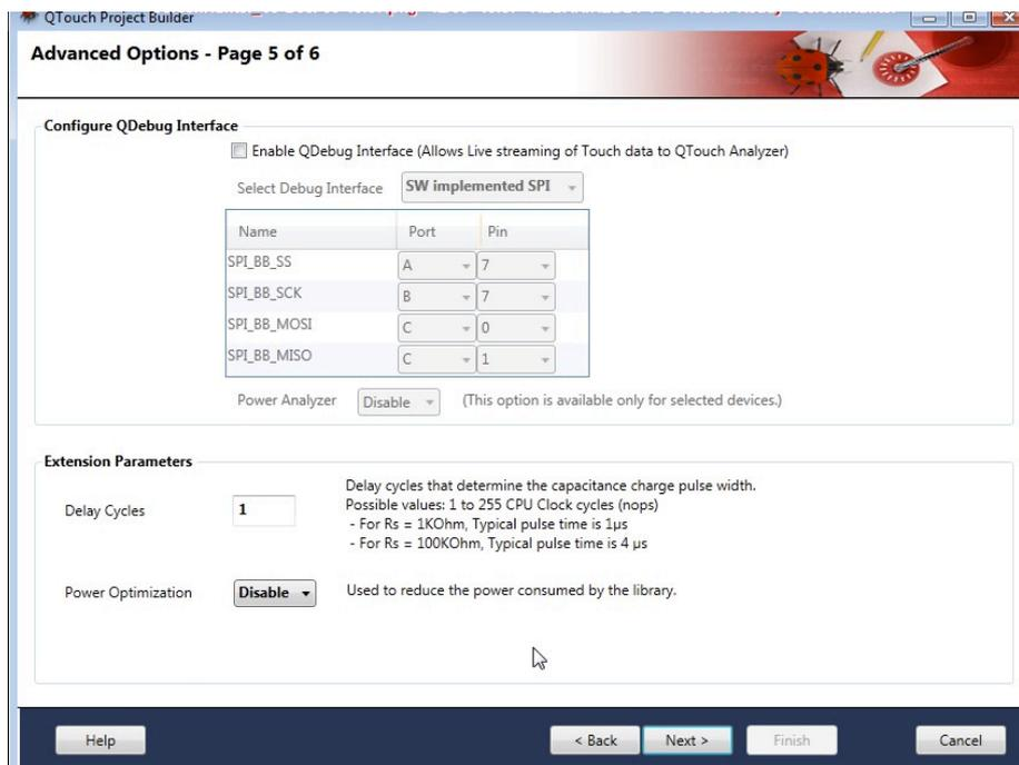
**Step 7 :** On clicking Next, a summary is generated. Click Finish. The wizard generates the code with separate files for setting up the timer, configuring the touch sensors, initializing the MCU system clock etc. There is also a main.c file that provides the user with an infinite loop to perform desired actions. The first step now is to configure the sensors using the function *config\_sensors()* in the file LED\_Blink.qtdgn → touch.c
