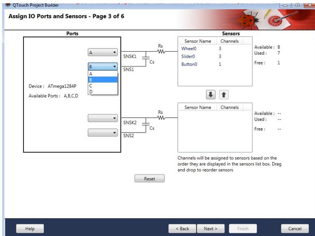
**Step 5 :** In this step, the exact Port pins have to be assigned to each sensor (as connected in hardware design). The pin numbers **HAVE** to be assigned in increasing order only. No sensor can have its channels connected to pins in decreasing order as mentioned before. However, it is not necessary that Port B pin 0 has to be connected to Port A pin 0; it can be any pin of A.
