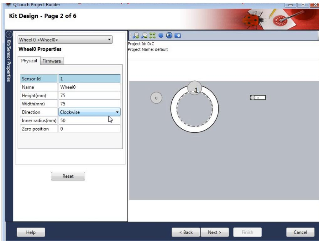
The sensor IDs are chosen as 0 for button, 1 for the wheel and 2 for the Slider.
