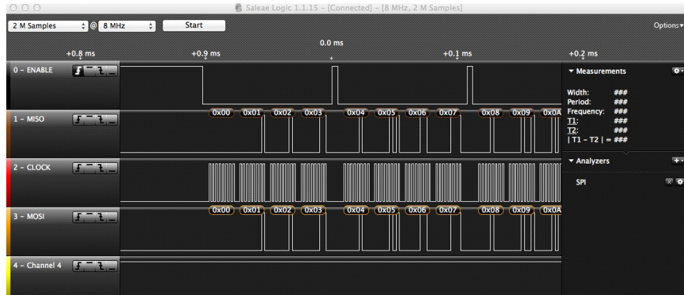
Figure 6.4: SPI Loopback Test Output
