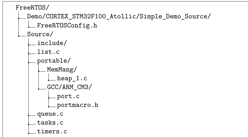
Figure 16.3: Key Parts of FreeRTOS Distribution
